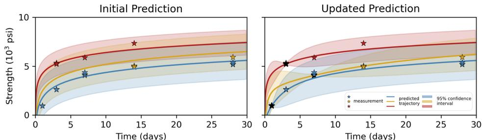
Figure 1: Strength trajectory predictions for three typical mixes from the test dataset using the GP model. *Left*: predictions using only the 13 mix descriptors. *Right*: predictions after observing one early strength measurement, denoted using a black star, for the same three mixes.
