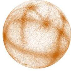
(a) Gauss map of the scanned data. Color opacity indicates confidence rate, the lighter in color the lower in confidence.
