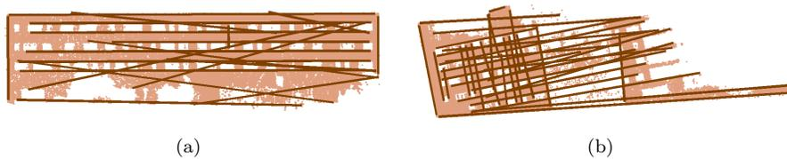
Figure 11: Spurious boundary lines are obtained due to window structure and occlusion.
