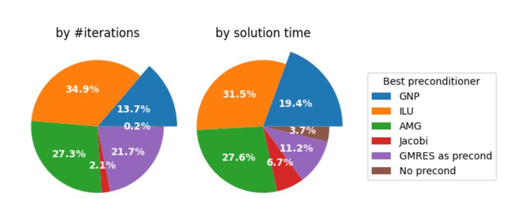
The construction time of GNP is predictable, while that of ILU and AMG is not. GNP sometimes is much faster to construct than ILU and AMG. GNP is faster in execution than GMRES as a preconditioner.
